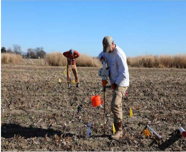
Drilling holes to install capacitance moisture sensors down to 48 inch at LTAR site, Stoneville, MS
