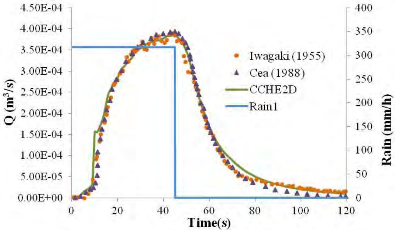
Figure 6: Runoff hydrograph for 2D validation test case 2B
