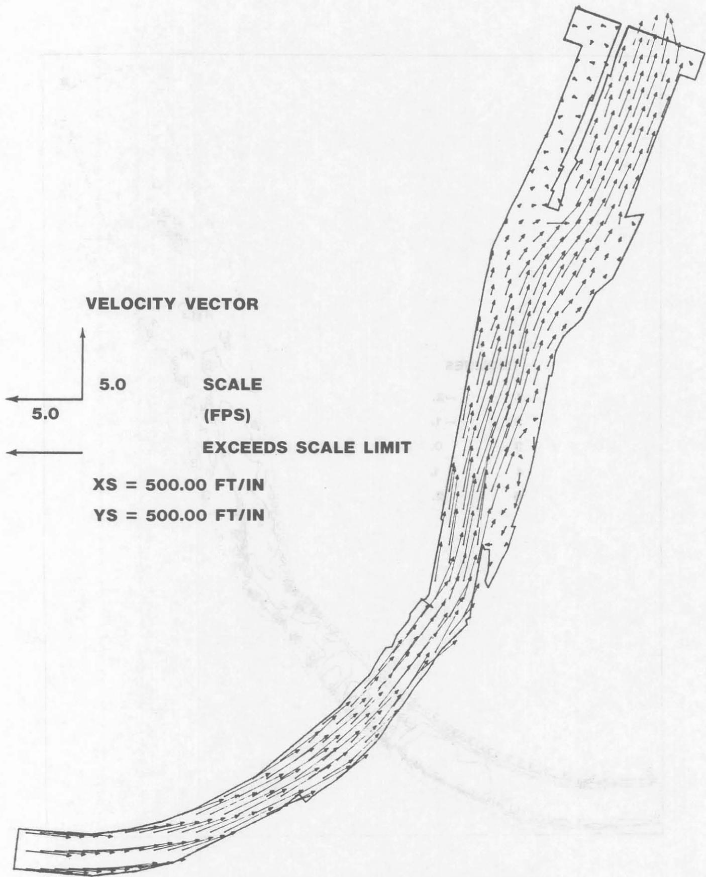
Figure 2 - Base condition velocity 40 ft pool 80000 cfs
