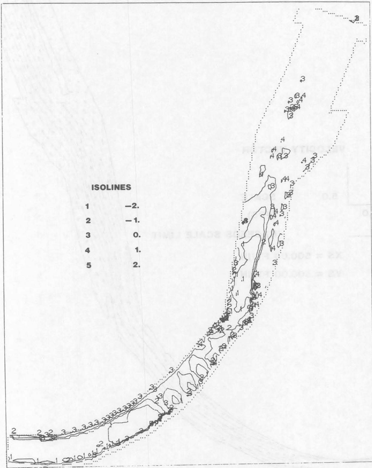
Figure 3 - Base condition bed change after STUDH simulation (M)
