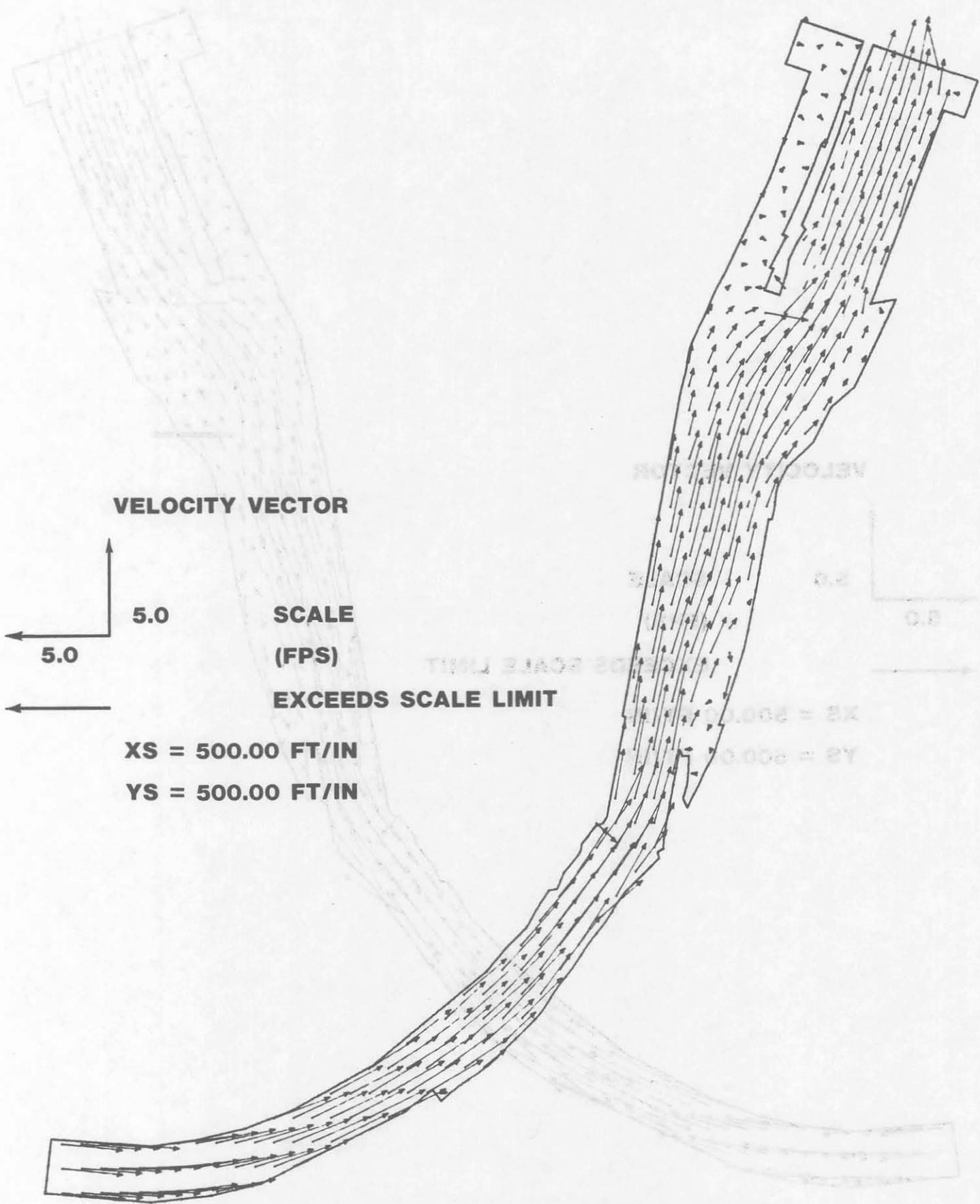
Figure 4 - Base condition velocity after STUDDH simulation
