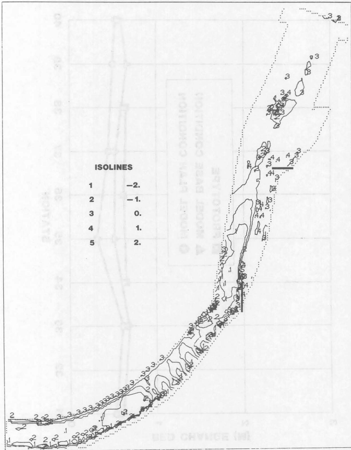
Figure 6 - Plan condition bed change after STUDH simulation (M)
