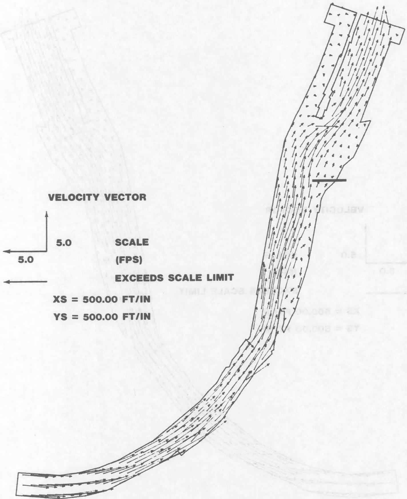
Figure 5 - Plan condition velocity 40 ft pool 80000 cfs
