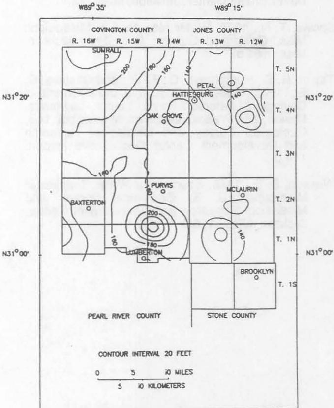
Figure 4. Computer-generated piezometric surface contour map for the shallow aquifer during the period 1984-1987.
