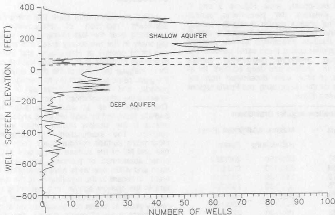
Figure 2. Histogram of water well screened interval versus number of wells showing approximate boundaries of the deep and shallow aquifers.
