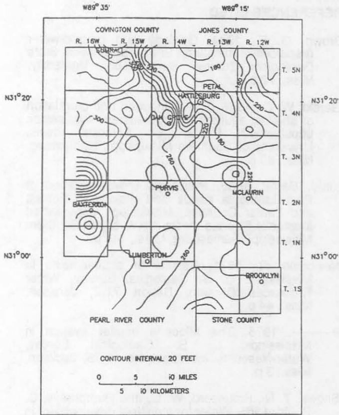
Figure 3. Computer-generated piezometric surface contour map for the shallow aquifer during the period 1960-1967.
