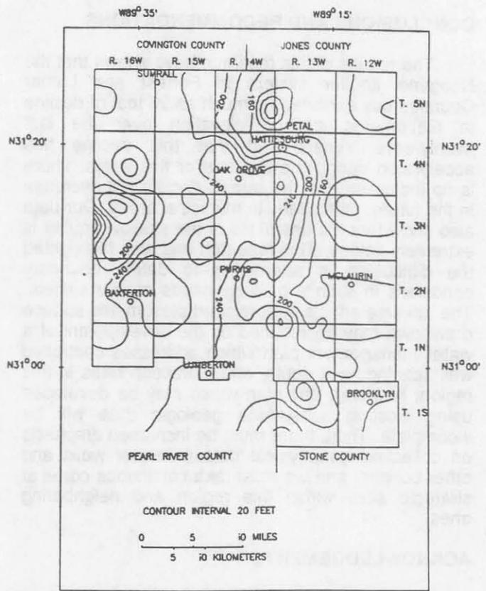
Figure 5. Computer-generated piezometric surface contour map for the deep aquifer during the period 1960-1967.
