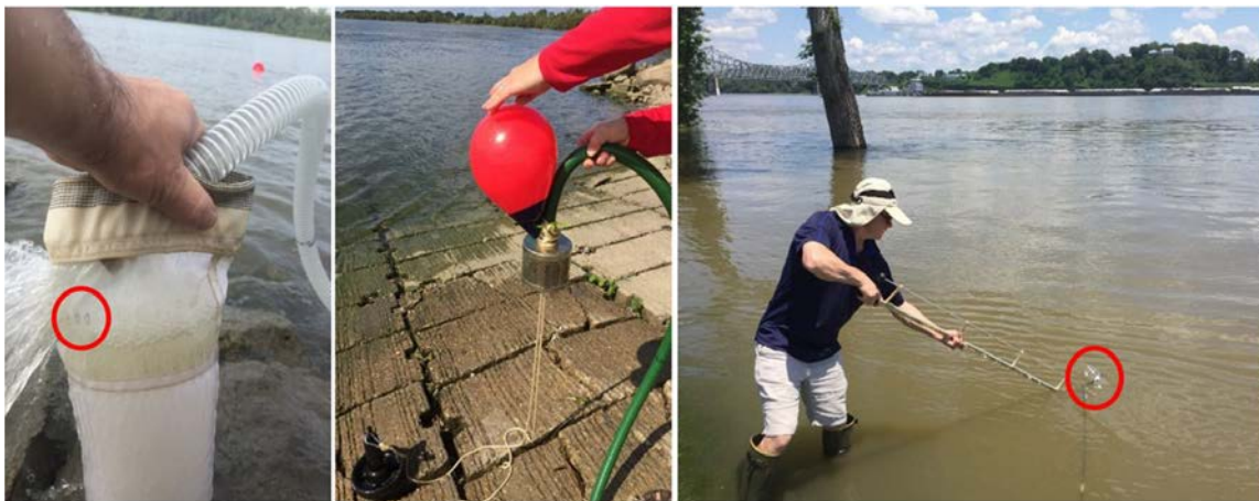
Figure 4. River water passing through the 100 \mu\text{m} cod-end net using the high-volume sampling method (left); intake chamber and hose for the high-volume sampling method (middle); and low volume grab-sampling with a ~ 1 L Mason jar.
