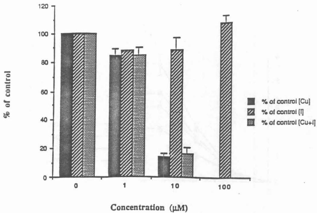
Figure 2. Effects of copper (II), imidazole, and their complex on mineralization of glucose in July California control ground water. Figure represents the mean  $\pm$  1 s.d.
