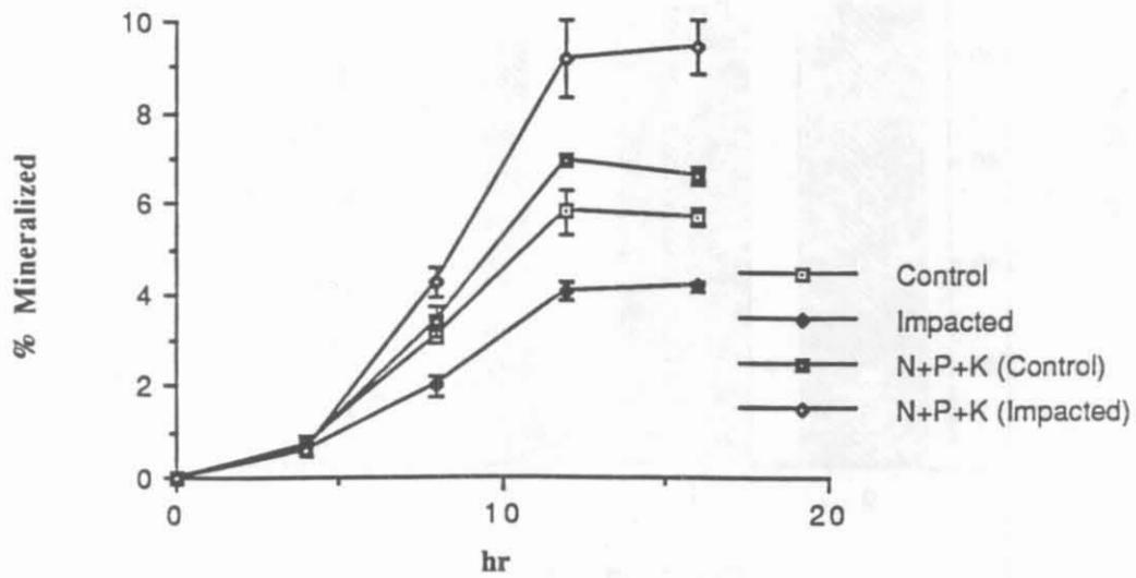
Figure 4. Effects of nutrients addition (N+P+K) on bacterial mineralization of phenol ( $1 \mu\text{g/liter}$ ) in California ground water. N & P were added at a final concentration of  $1 \text{ mg/liter}$ ; K was added at a final concentration of  $4 \text{ mg/liter}$ .
