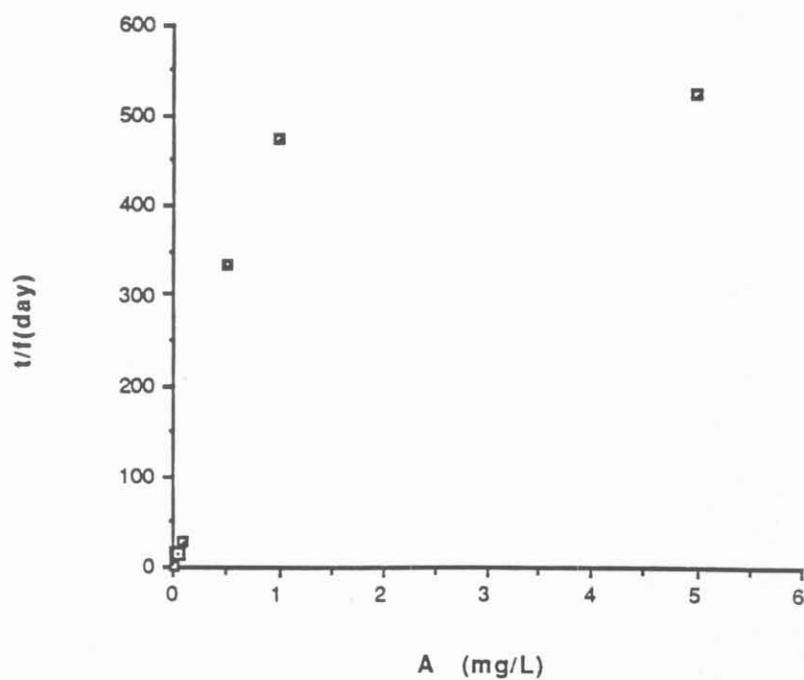
Figure 3. Wright-Hobbie plot for p-cresol mineralization in Georgia control ground water.
