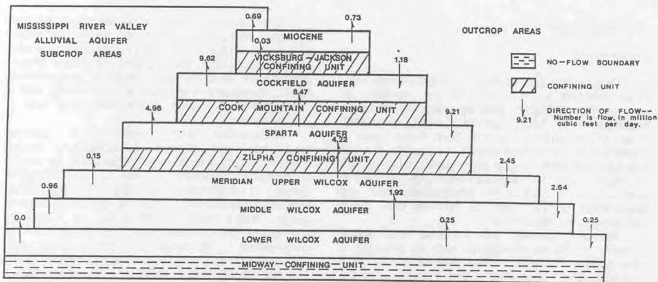
FIGURE 9. SUMMARY OF MODEL SIMULATED FLOW ASSUMING PREDEVELOPMENT CONDITIONS.
