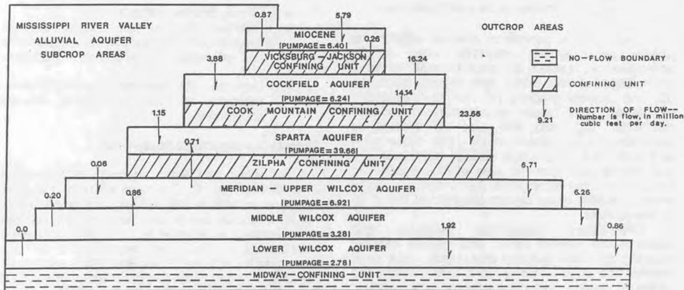
FIGURE 10. SUMMARY OF MODEL SIMULATED FLOW ASSUMING 1980 PUMPAGE CONDITIONS.
