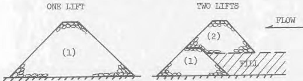
FIGURE 17 - CONSTRUCTION BY LIFTS ON POINT BARS
