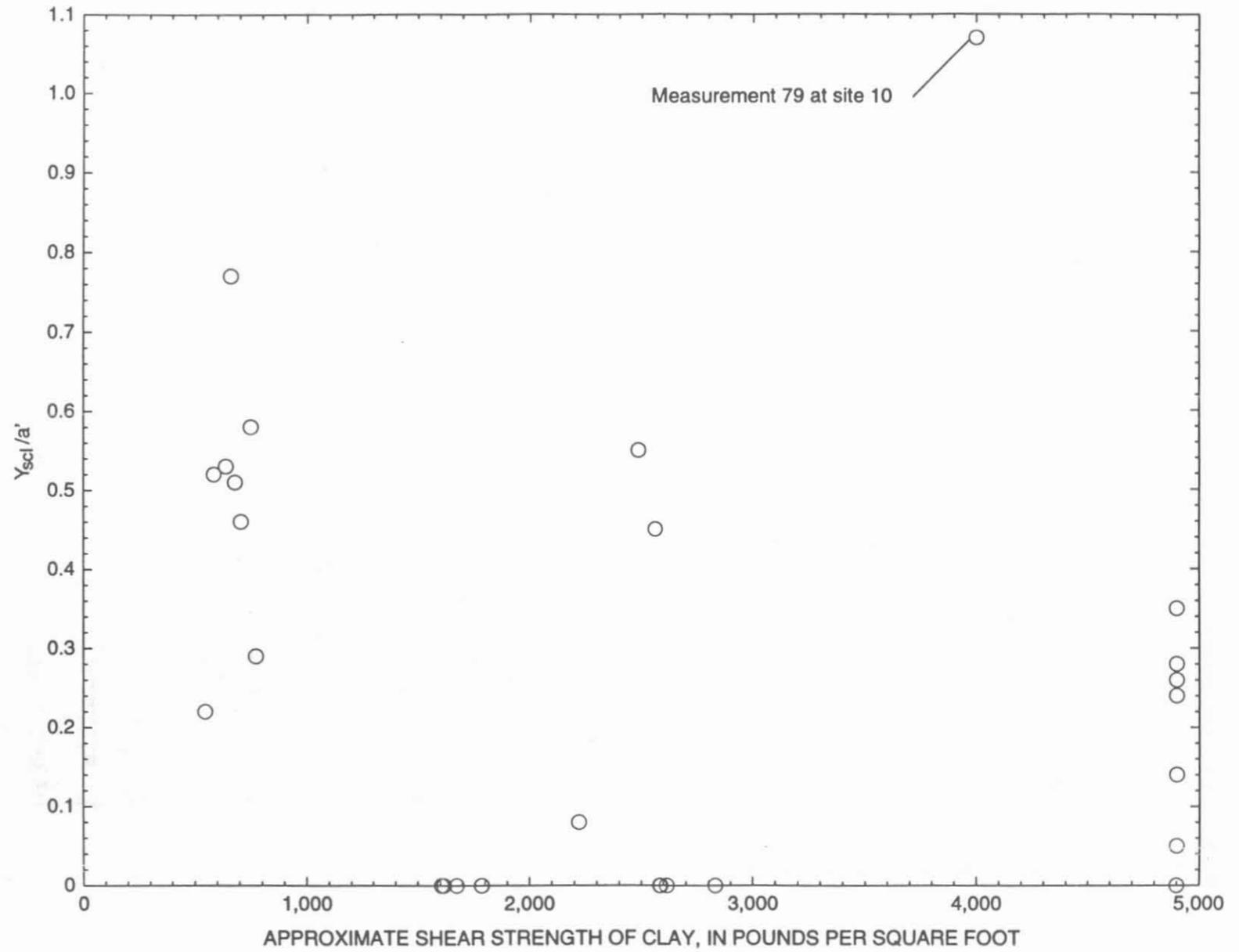
**Figure 4.** Relation between net pier-scour depth through clay divided by normal pier width ( $Y_{scl}/a'$ ) and approximate shear strength of clay for selected bridge sites in Mississippi.
