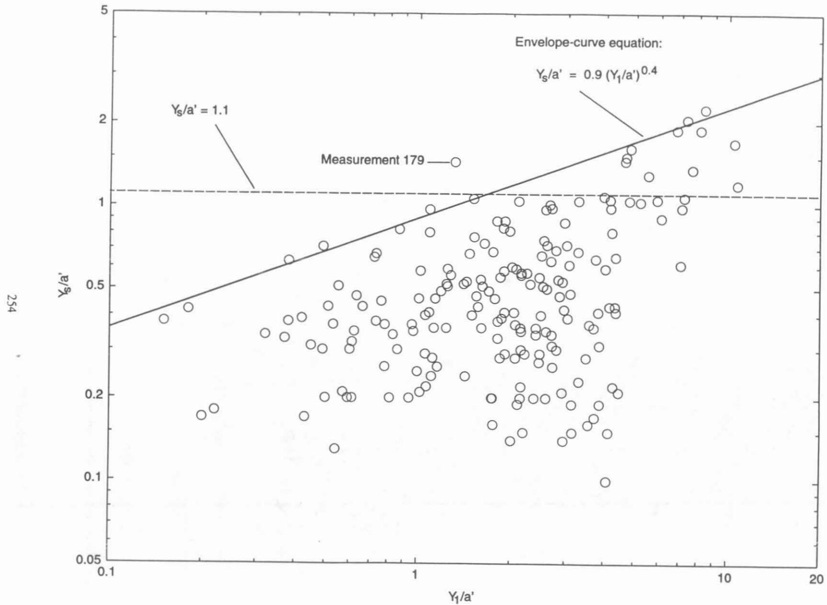
**Figure 2.** Relation between measured pier-scour depth divided by normal pier width ( $Y_s/a'$ ) and measured approach-flow depth divided by normal pier width ( $Y_1/a'$ ) for selected bridge sites in Mississippi.
