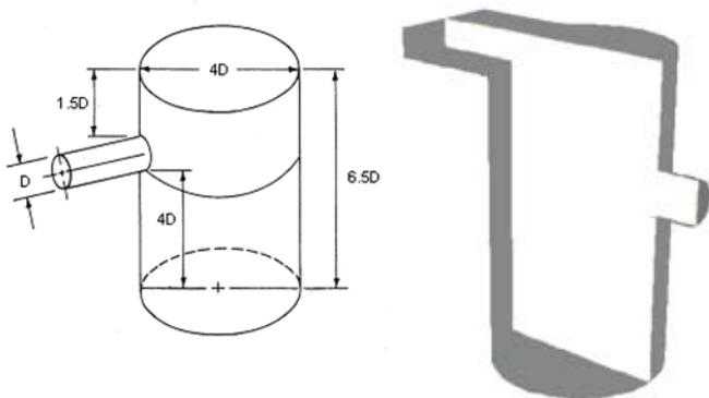
Figure 1. Typical catchbasin geometry by Larger, et al. (1977) (left) - 2D longitudinal center-line cross section (right).
