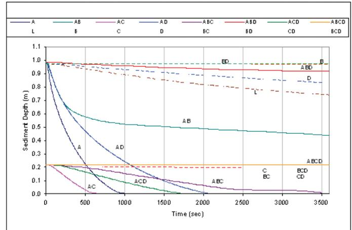
Figure 3. Reduction of Sediment Depth as a function of Time for each treatment. Results of the  $2^4$ -full factorial experiment (A: flow rate; B: particle size; C: water depth; and D: specific gravity).
