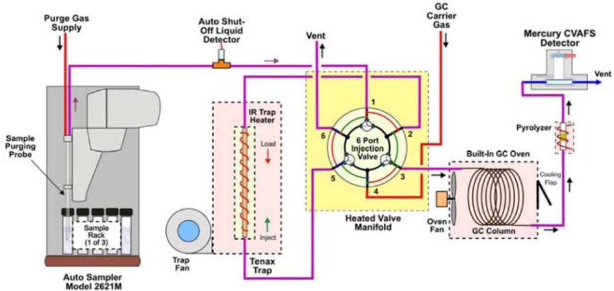
Figure 3. Flow diagram for the methylmercury analyzer (Tekran 2700).
