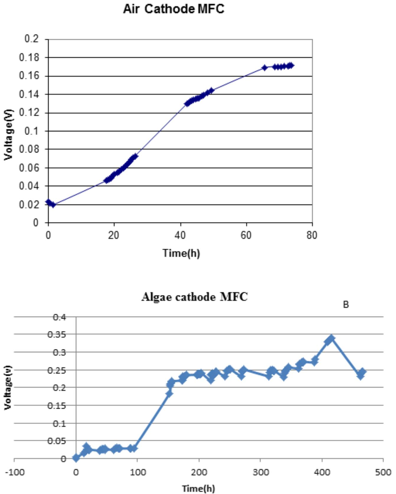
Figure 2 Voltage profile for air cathode MDC and Algal cathode MDC
